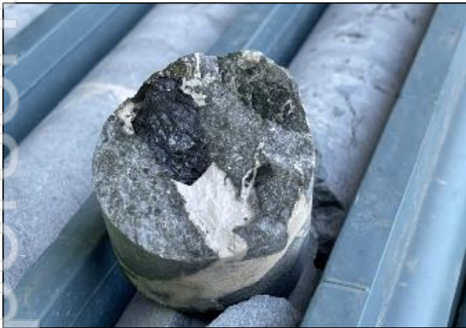
Figure 10. Photo of diamond NQ drill core showing sphalerite (black) and wollastonite (white) infill in section of brecciated sandstone from MPD003. ØNQ drill core.
