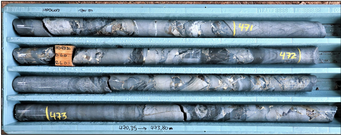
Figure 11. Representative section of brecciated core from MPD003 showing both sandy units (lighter greys) and mud-rich units (dark grey). The host low-grade metasediments are heavily brecciated and show infill with predominantly quartz and carbonate together with sulfides, mainly pyrite with sphalerite and minor galena in MPD003. The metasediments also exhibit fine network veining with sulfides as well as disseminated sulfides throughout. Core is NQ from 470.35m to 473.80m down hole. The average silver grade is 10g/t Au from sample MPDN470 (470-471m) to sample MPDN473 (473-474m).
