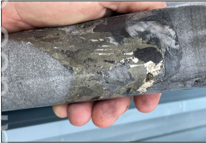
Figure 9. Photo of NQ drill core showing pyrite, sphalerite, wollastonite and quartz infill in the brecciated section of sandstone. MPD003 ØNQ drill core
