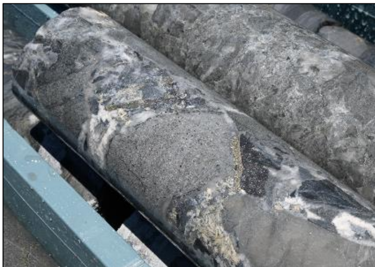
Figure 3. Photo of brecciated sandstones with infill containing sulfides pyrite, sphalerite, and galena. ØHQ drill core.
