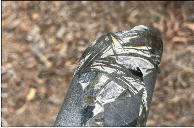
Figure 8. Wollastonite, pyrite, and sphalerite infill in brecciated sandstone and mudstones. MPD003 ØNQ drill core.
