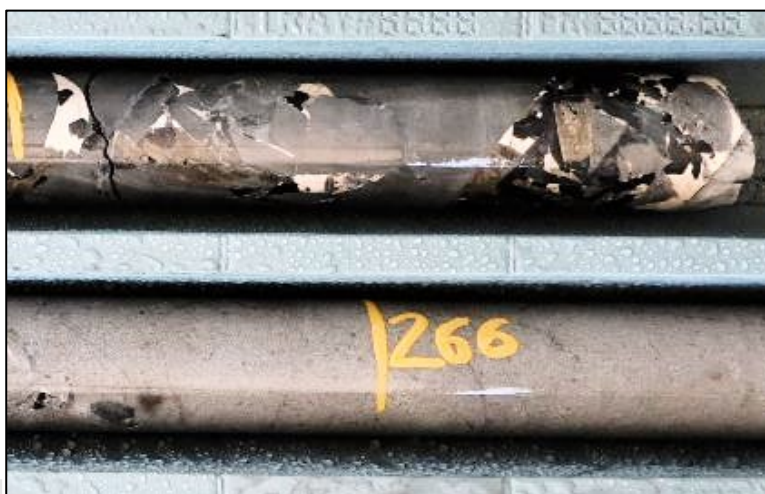
Figure 4. Section of drill core at 265-265.25m containing abundant sphalerite in fragmented (brecciated) mudstone. ØNQ drill core.
