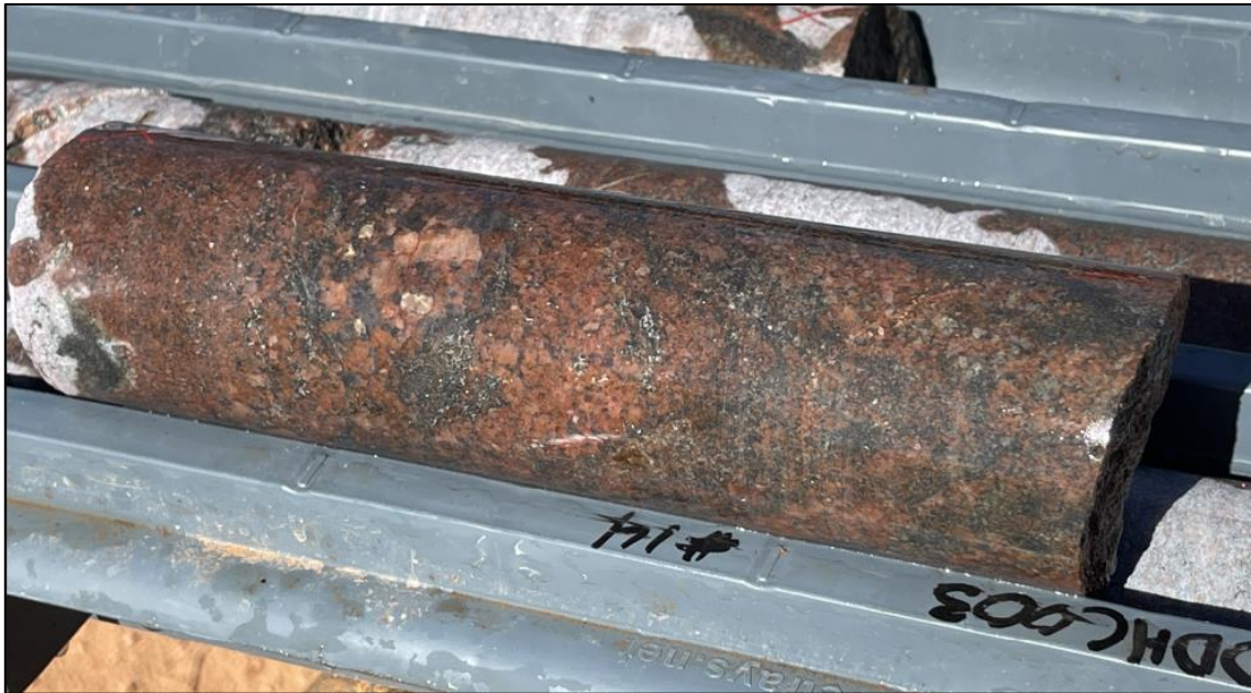
Figure 6: altered granite in HQ drill core from Central_DD003. The granite contains minor hematite staining, secondary biotite, pyrite and magnetite.
