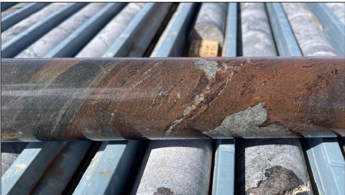
Figure 4. Photo of HQ diamond drill core CENTRAL_DD003 showing hematite staining of country rocks.
