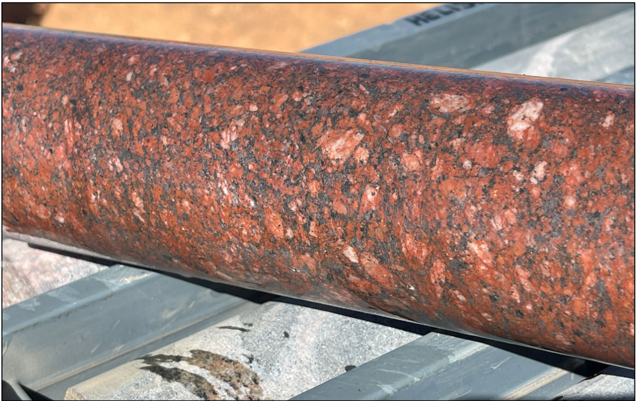
Figure 2. Image of the first samples of HQ diamond drill core from Helios_DD002. The drill core is HQ diameter and shows pervasive alteration of the host granite.
