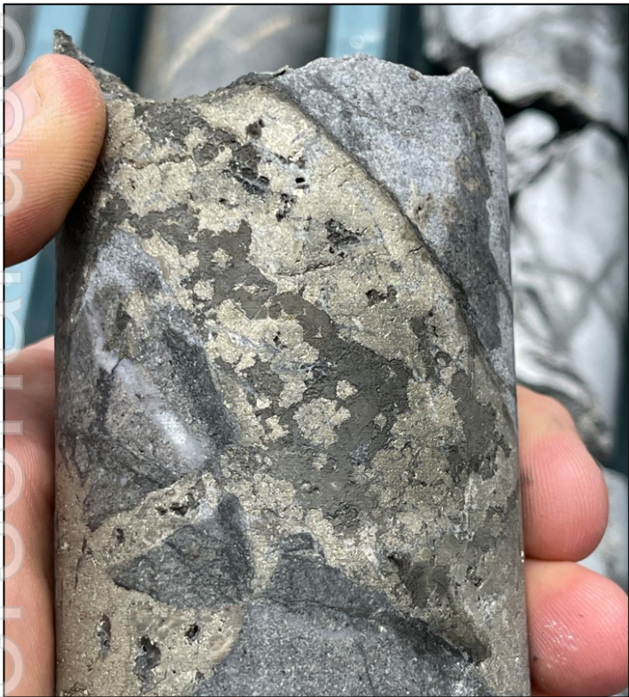
Figure 5. Section of HQ3 drill core from MPD003 between 100 and 110m depth showing massive sulfide infill between breccia fragments.
