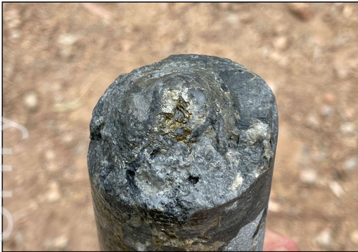
Figure 4. Section of HQ3 drill core from MPD003 containing chalcopyrite and pyrite infill between metamorphosed and altered host sandstones (meta-sandstone protolith).
