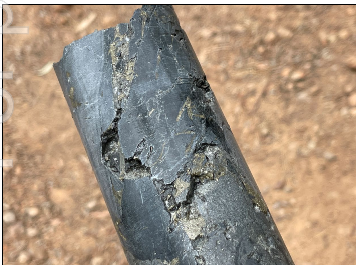
Figure 6. Section of HQ# drill core from MPD003 between 100 and 110m showing the characteristic open space cavities in the brecciated rock. The cavities are common in all rocktypes and show infill with sulfides including cubic pyrite crystals.
