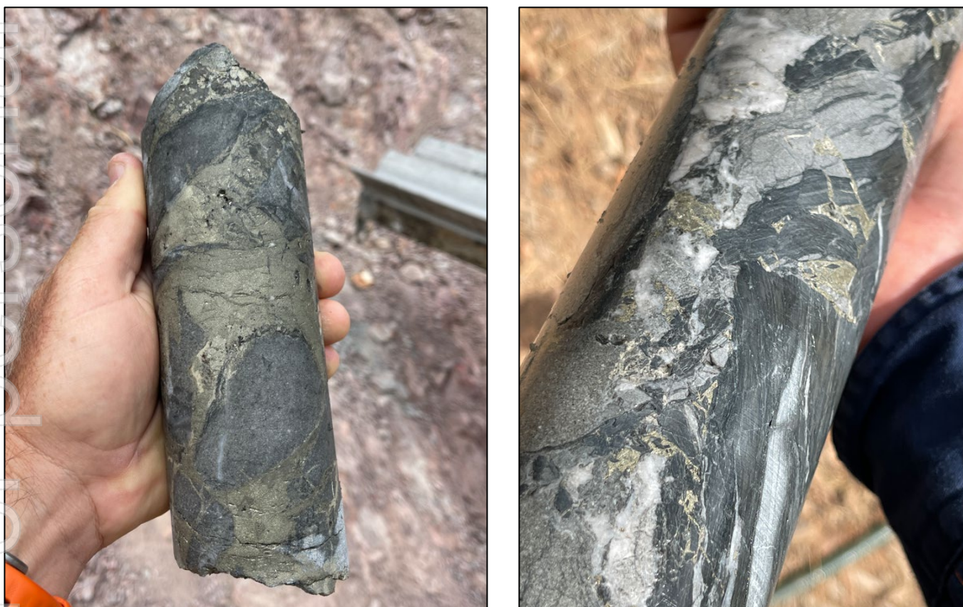
Figure 2. Photos of sulfides and quartz + sulfides in-filling breccia fragments. Host rocks are altered metasediments. Sulfides include pyrite, chalcopyrite, sphalerite +/- galena. (MPD003 - HQ3 diameter drill core).
