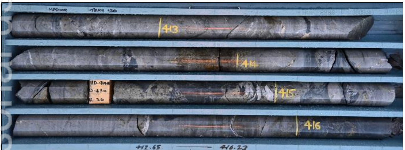
Figure 1. Section of drill core (414-415m) containing 57.1 g/t Ag, 0.1 g/t Au, 0.51% Zn, 0.12% Cu, 0.23% Pb and 204 g/t Sb.
