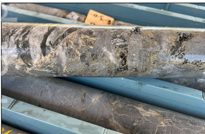
Figure 8. Abundant network veining of sulfides amongst breccia fragments in a sandstone (low-grade metamorphosed) with small amounts of darker mustone, which referentially fracture and contains the majority of sulfides and sulfide-mineral assemblages.
