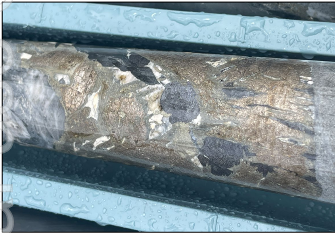
Figure 10. Photo of diamond HQ drill core showing a similar variety of sulfides but an abundance of sphalerite which was common in MPD003 relative to MPD002.
