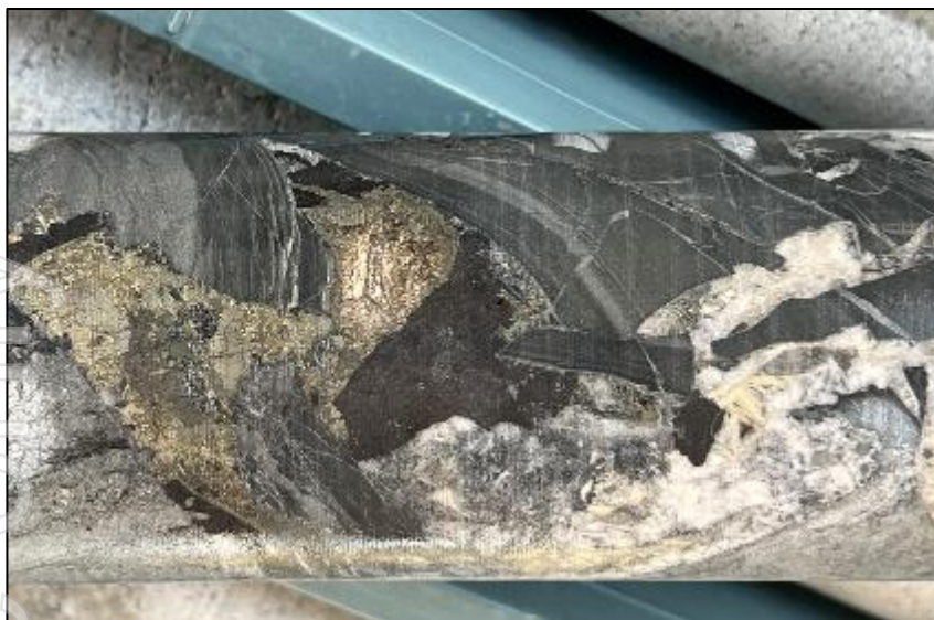
Figure 2. Photo of brecciated mudstone (pelite) showing original depositional bedding/layering. The fragments are broken, rotated and the infill space replaced with sulfides (mainly pyrite and sphalerite), quartz and carbonates. MPD002 approx. 284.3m down hole depth. ØHQ drill core.
