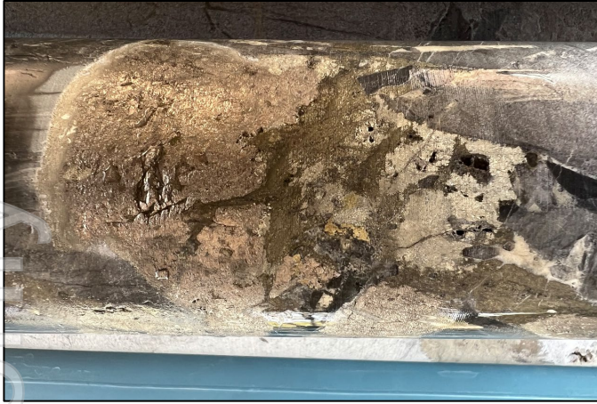
Figure 9. Photo of HQ drill core showing the variety of sulfides including pyrite pyrrhotite, sphalerite.
