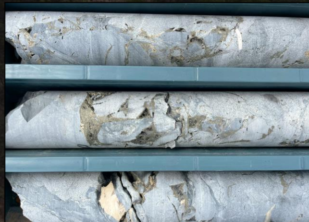
Section of HQ drill core showing cavities with some sulfide infill between breccia fragments. MPD003 HQ3 diameter drill core between 110 and 118m.
