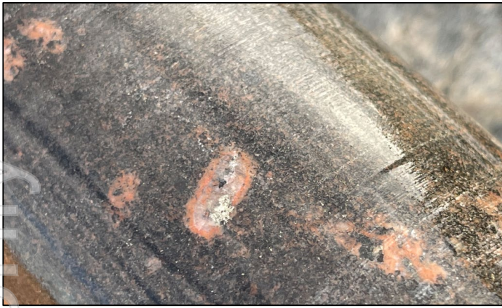
Figure 15. Image fo NQ ½ drill core HELIOS_DD002 showing K-feldspar phenocryst in fine grained diorite. The already altered phenocryst shows partial replacement by pyrite.
