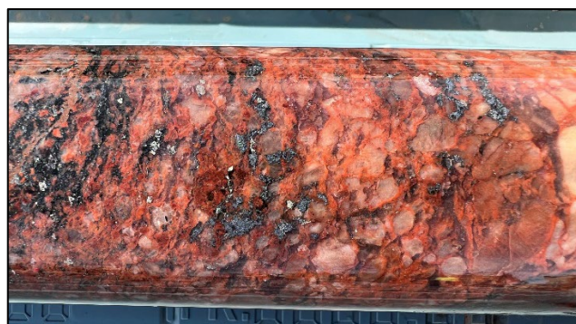
Moderately altered granite from HELIOS_DD001 (ØNQ). An example of heavily altered granite is provided in figures 1 and 2.
