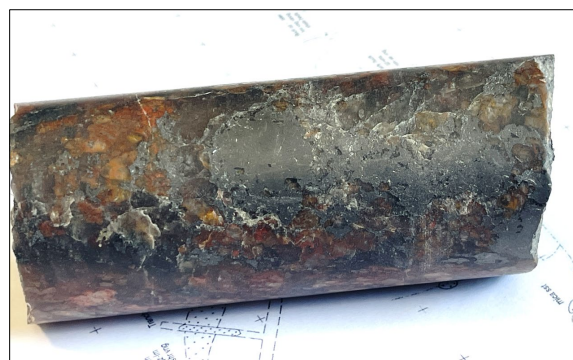
Figures 1 and 2. Photos of NQ drill core with some examples of hematite (grey mineral in left image) and magnetite (grey mineral in right image) replacing the granite groundmass. Hematite staining (red) in both samples is pervasive, however, the image on the left is an example of where the host granite has been almost completely overprinted by hematite staining to the point where the host rock is difficult to recognise. Drill core is ØNQ, HELIOS_DD001.
