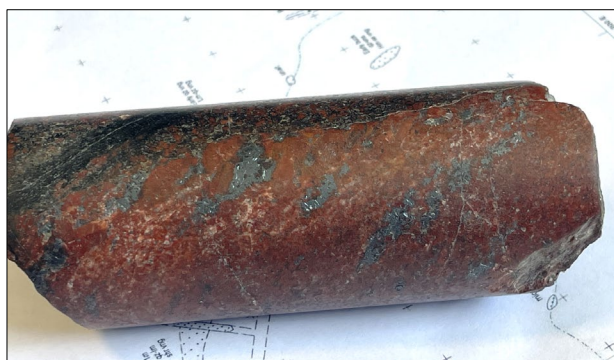
Figures 1 and 2. Photos of NQ drill core with some examples of hematite (grey mineral in left image) and magnetite (grey mineral in right image) replacing the granite groundmass. Hematite staining (red) in both samples is pervasive, however, the image on the left is an example of where the host granite has been almost completely overprinted by hematite staining to the point where the host rock is difficult to recognise. Drill core is ØNQ, HELIOS_DD001.
