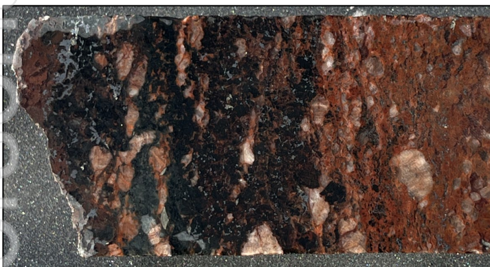
Figure 13. Image fo NQ 1/2 drill core HELIOS_DD01 showing a range of alteration minerals and textrues. Red alteration is hematite staining of host granite and replacement of groundmass. Part of the rock is also replaced by biotite, amphibole and hematite. The host granite is almost unrecongnisable in this part of the drill core due to the pervasive multi-phase alteration.
