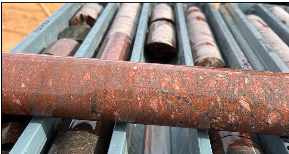
Figure 5. Pervasive iron oxide staining and hematite in altered granitic host rocks (HELIOS_DD002).
