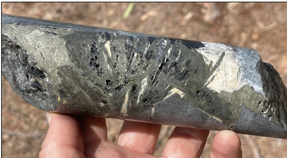
Figure 1. Photo of semi-massive sulfides from drill hole MPD003. Sulfide components are pyrite and sphalerite together with wollastonite in brecciated sandstone. Drill core is \emptyset NQ.
