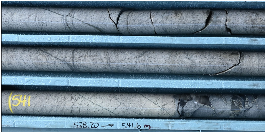
Figure 3. Section of drill core showing the heavily phyllic altered porphyry containing minor sulfides as replacements, disseminated and in abundant small crossing veins. The contact with host low-grade brecciated sediments containing pyrite and sphalerite and carbonate (wollastonite) in matrix is present in the bottom right. Depth of contact is 541.3m down-hole.
