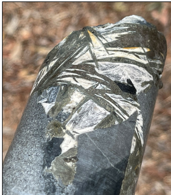
Figure 2. Spectacular bladed pyrite and sphalerite replacing or inter-grown with bladed wollastonite in brecciated sandstone fragments. Core is ØNQ. Depth of sample is 164m.
