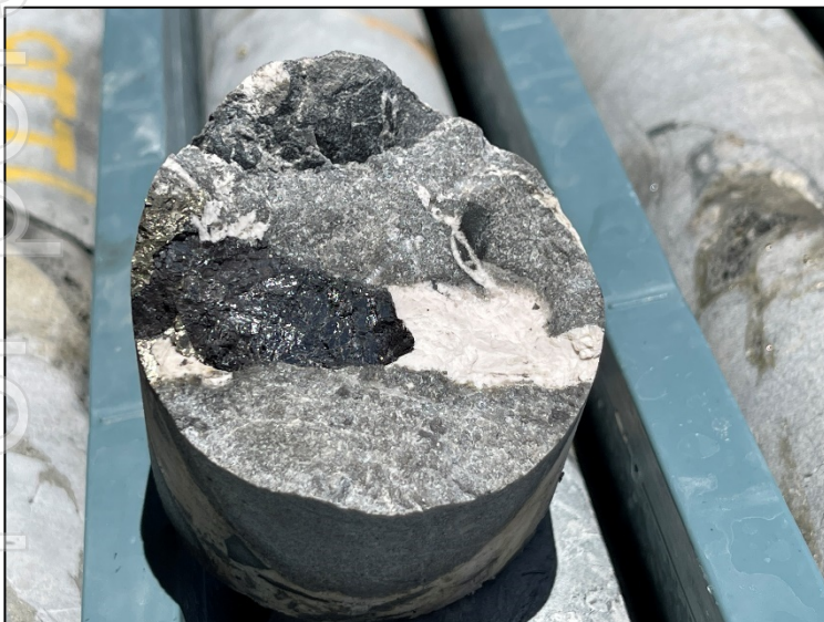
Figure 5. NMR are continuing to recover spectacular sulfide-bearing breccias from drill hole MPD003. The current drill hole is at 145m depth. Sample shows sphalerite with pyrite in carbonate vein cutting host metasandstone which also contains abundant disseminated sulfides.
