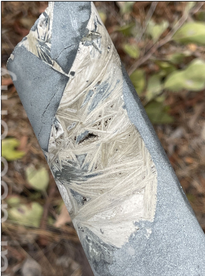
Figure 4. Section of ØNQ drill core from MPD003 (183.4m) containing wollastonite and sphalerite+pyrite between metamorphosed and altered host sandstones (meta-sandstone protolith). Wollastonite is (CaSiO 3 ) a good indicator mineral for skarn-type mineral deposits including the nearby Chillagoe deposits (e.g. Redcap) where Wollastonite forms part of a prograde skarn assemblage.
