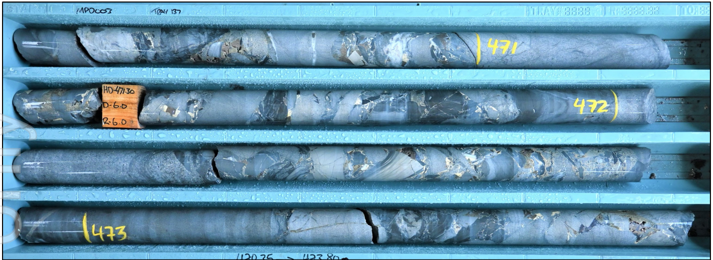
Figure 7. Just a few examples of the amazing, brecciated rocks being recovered in drill core from the Maneater prospect. Meter-long sections of core typically contain approximately 5% semi-massive or massive sulfides but the rocks contain pervasive disseminated sulfides and abundant cross-cutting sulfide bearing mm-scale stringer veins which are difficult to capture in images of core at this scale.
