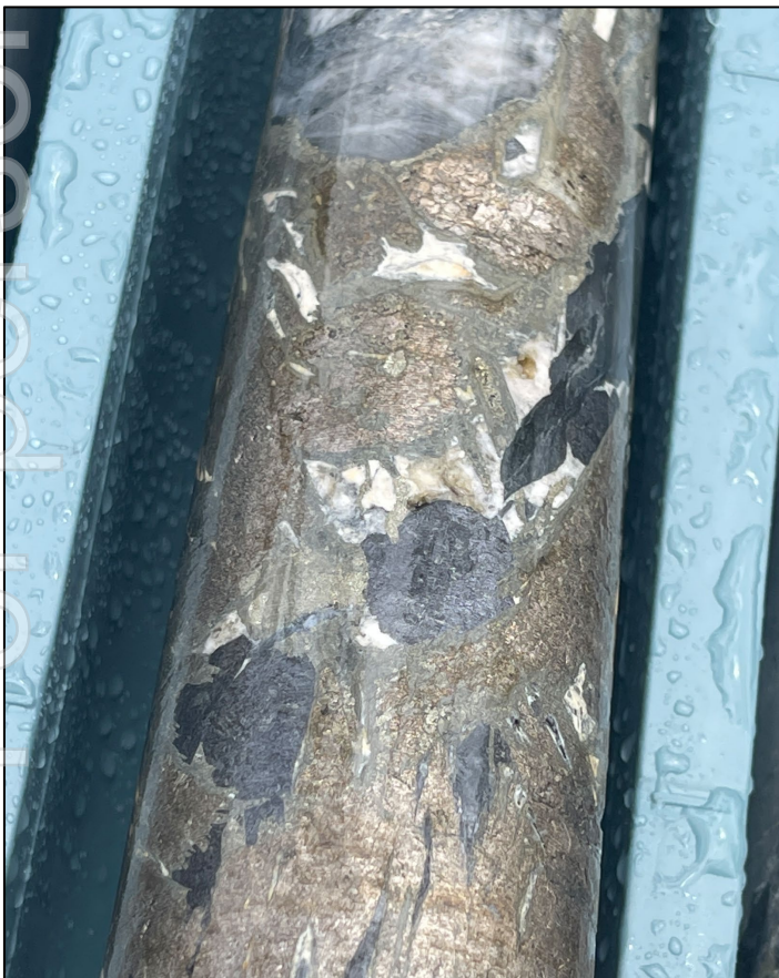
Figure 5. Section of ØNQ drill core from MPD003 depth showing semi massive sulfide (pyrite and sphalerite) infill with wollastonite between breccia fragments.
