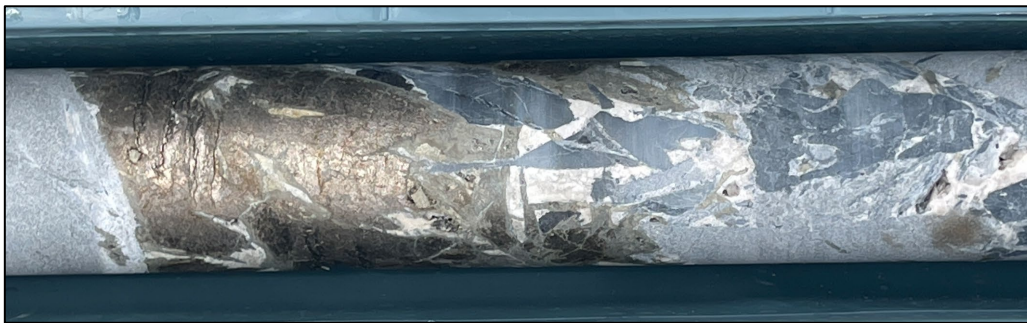
Figure 4. Photos of sulfides at 185.5m in-filling breccia fragments. Host rocks are altered metasediments. Sulfides include predominantly pyrite and sphalerite. (MPD003 – NQ diameter drill core).
