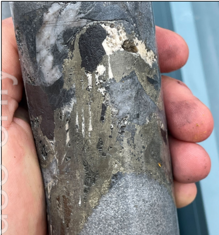
Figure 6. Section of ØNQ drill core from MPD003 from a depth of approximately 368m down hole. Quartz infill with sphalerite, pyrite and carbonate between low-grade metamorphosed sandstone fragments.
