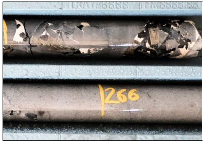
Figure 4. Section of drill core at 265-265.25m containing abundant sphalerite in fragmented (brecciated) mudstone.
