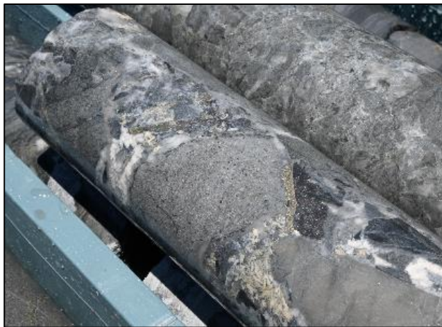
Figure 3. Photo of brecciated sandstones with infill containing sulphides pyrite, sphalerite, and galena.
