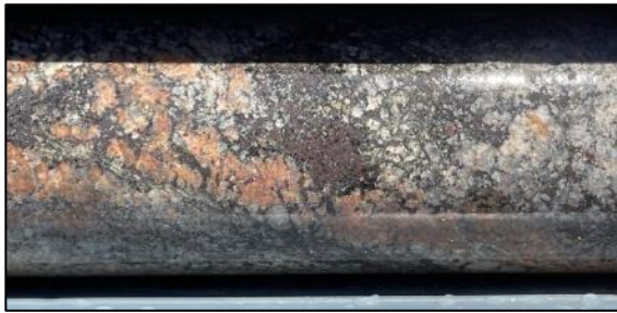
Figure 18. Photo showing an example of granite found in drill core from Central DD003.
