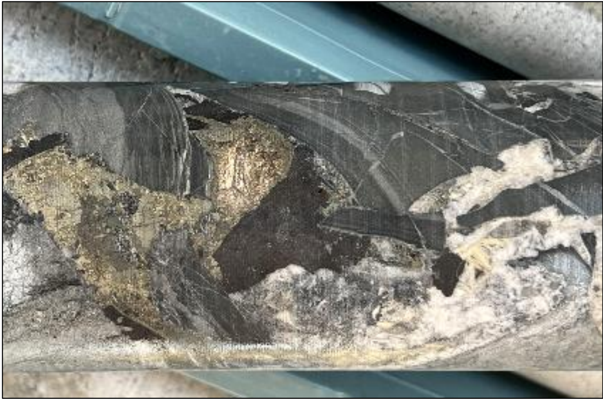
Figure 3. Photo of brecciated mudstone (pelite) showing original depositional bedding/layering. The fragments are broken, rotated and the infill space replaced with sulfides (mainly pyrite and sphalerite), quartz and carbonates. MPD002 approx. 284.3m down hole depth. ØHQ drill core.
