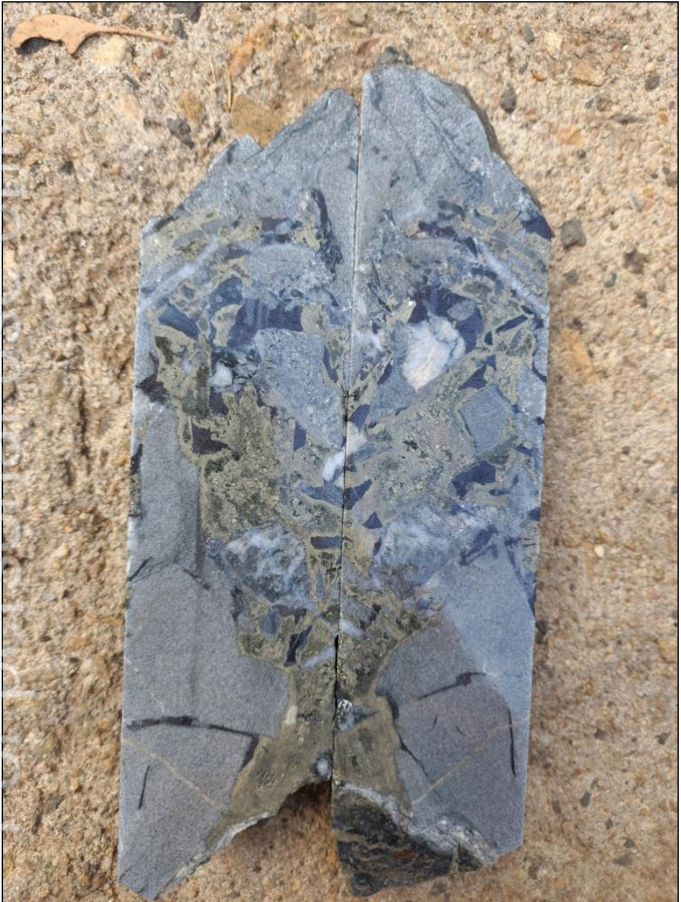
Figure 7: Section of MPD005 core displaying breccia with massive pyrite & sphalerite (black material) mineralisation (276.6m)
